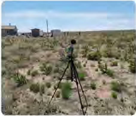
The assessment of traffic noise from the proposed project was determined from measurements obtained using a sound level meter.
