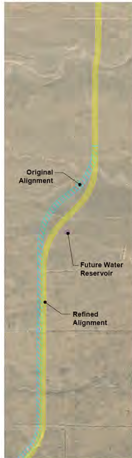
Figure 5-4. Realignment of Reverse Curves in Middle Section
