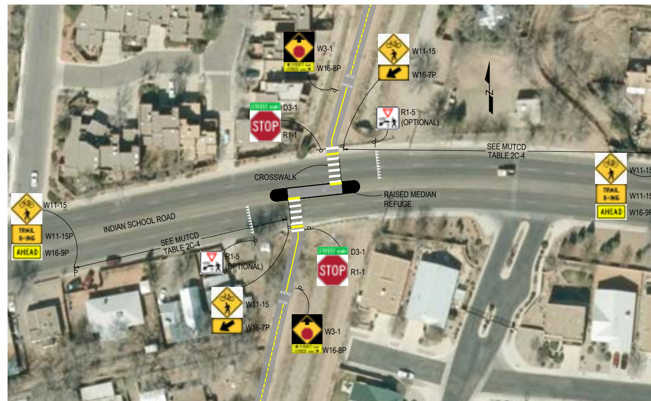
FIGURE 28. Mid-Block Crossing - Indian School Road
